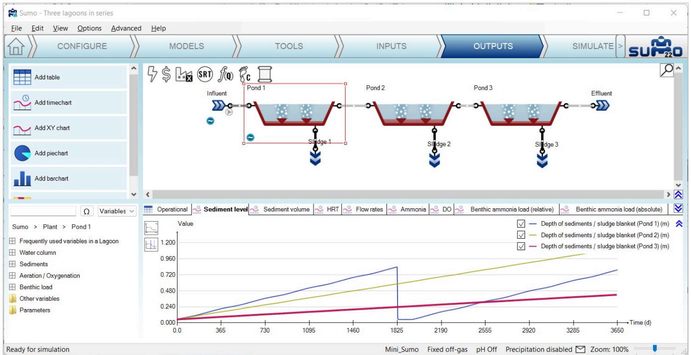
Figure: Simulation of pond sediment depth accumulation with desludging event after 5 years
